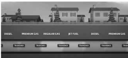
PIPELINE COMPANIES USE BATCHING LINES
